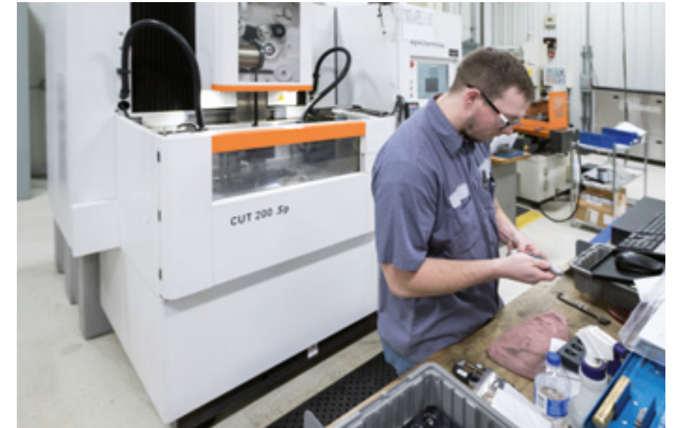
Micropulse's AgieCharmilles CUT 200 Sp wire EDM allows the shop to generate parts to micron tolerances, especially those with variable heights.
