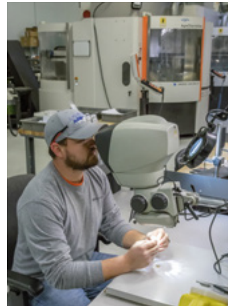
Some of the surgical implants Micropulse produces on its GF Machining Solutions machines are so small and intricate that inspecting them requires special magnification systems.
