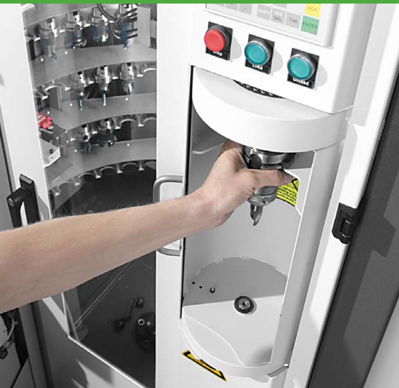
Circular magazine design with handling system
