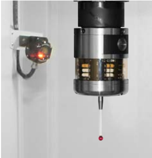
Touch probe radio RMP 60
