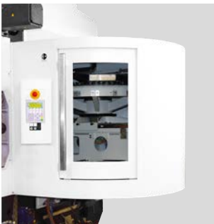
Tool magazine HSK-A/T100: 30 tools HSK-A/T63: 45 tools
